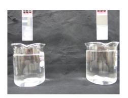
Apply each sample at 0.2g/cm<sup>2</sup> on a glass plate and dry well, then soaked in water with gentle stirring
